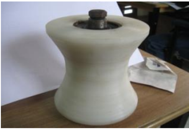
CABLE GUIDE ROLLER FOR HMC
