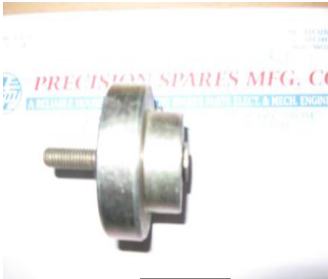
Moving roller with lock of VCB;
