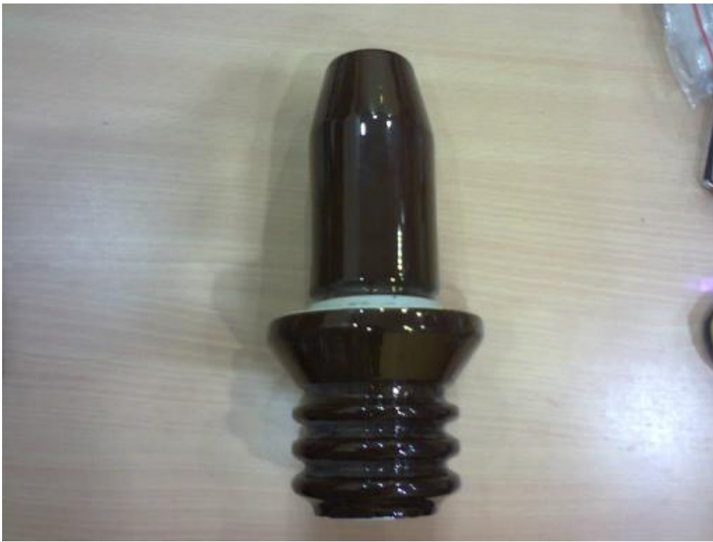
11 Kv bushing porcelain insulators
